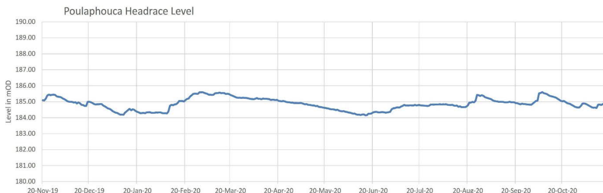
Figure 5. Poulaphouca Headrace Water Levels
